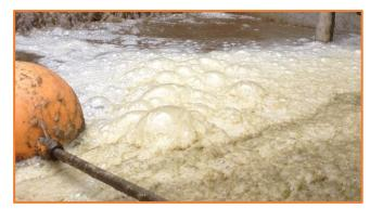
Effective foam control requires accurate data on foam behavioural parameters in real time. However, the effective and reliable measurement of foam thicknesses and foam-liquid interfaces presents a number of challenges. Traditional measurement techniques have been based on a range of existing level probe technologies 'adapted' for foam measurement. In most applications these tend to be inherently unreliable, inaccurate and adversely affected by process product build-up on the measuring probes.
